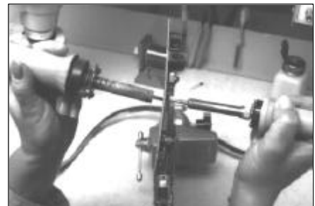
Figure 2: Place a soldering iron tip against the component lead and the desoldering tip over the lead end.
