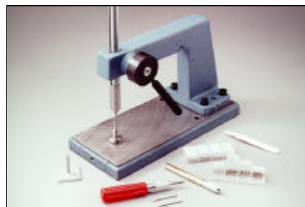
Figure 2: Set the eyelet using an Eyelet Press System.
