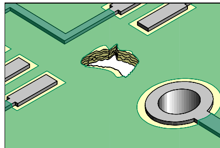
Damaged Base Material
